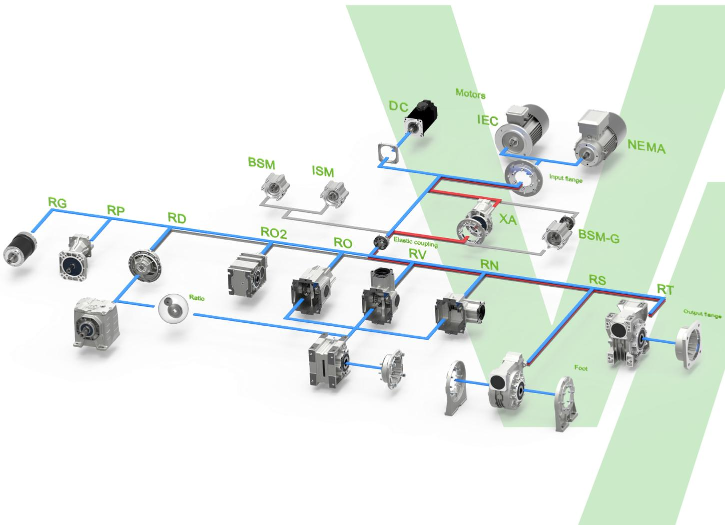
The RS and RT Series of worm gearboxes are designed to be the ideal solution for applications that require small or medium power ratings for their drive.
